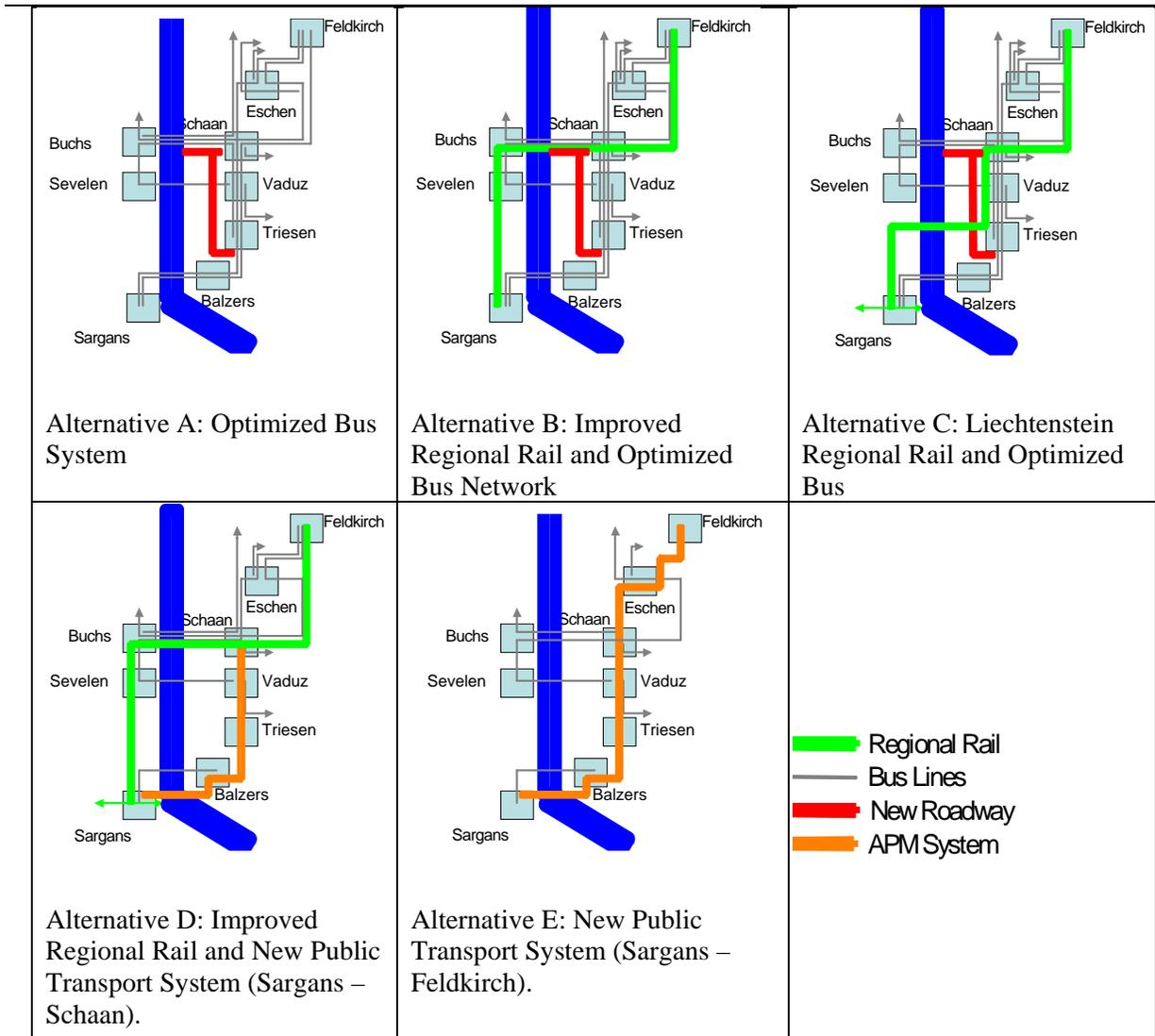
**Figure 3: Schematic Diagram of Alternatives; arrows show ongoing lines**
