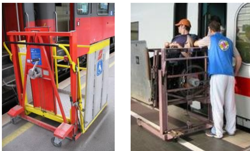
Figure 4: Platform-based manual lift.
