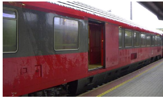
Wide doors on existing baggage car.
