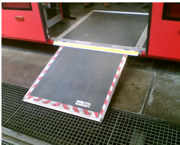
Figure 3: Vehicle-based automatic ramp.
