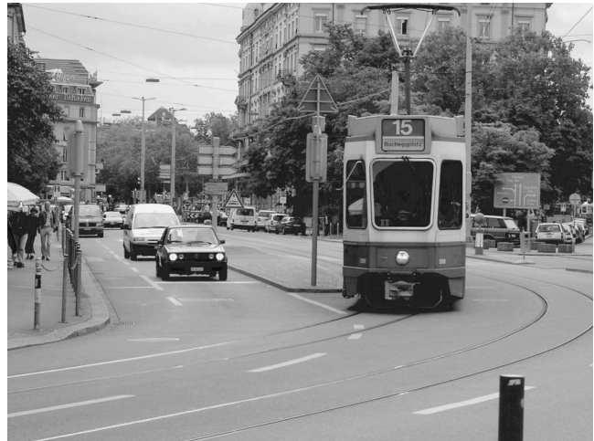
FIGURE 2 Transit priority provided by traffic signal—traffic signal stops private traffic, enabling tram to go first as it moves from separate right-of-way to shared right-of-way.
